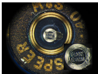
The primer has been stamped by the firing-pin.
