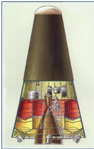
Figure 19: Sectional view of the upper section of the R36-O, showing the engine used to place the 8F673 nuclear payload into orbit (Credit: Christian Lardier)
