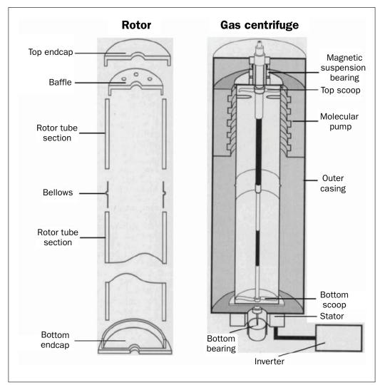
Figure 3.2. Basic gas centrifuge design
