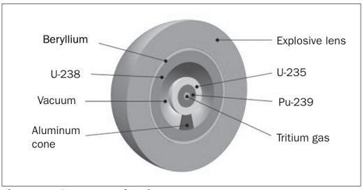
Figure 3.1. Basic components of a nuclear core
